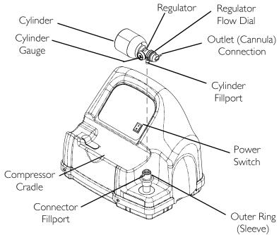
NOTE: Cylinder bag, cylinder fillport cover and connector fillport cover are not shown for clarity.
